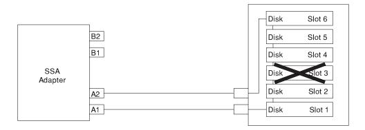
If two or more disk drive modules are turned off, fail, or are removed from the loop, some modules might become isolated from the SSA adapter.
